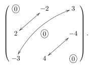
The elements located at the ends of the same arrow must be opposites and those on the diagonal (enclosed in a circle) must be zero.
