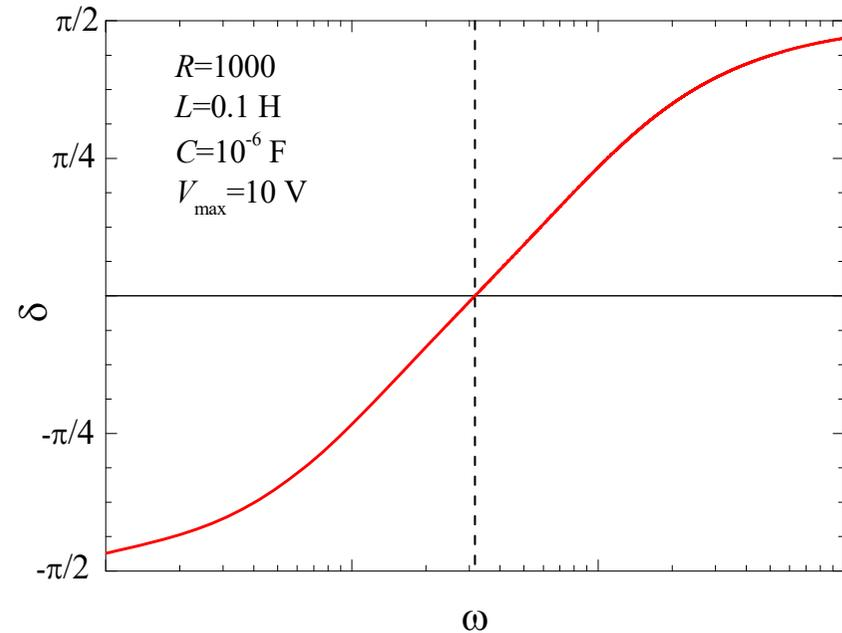
$$I_{\max} = \frac{V_{\text{app}}}{R} \quad \omega_{\text{res}} = \frac{1}{\sqrt{LC}} \quad \delta = 0$$
