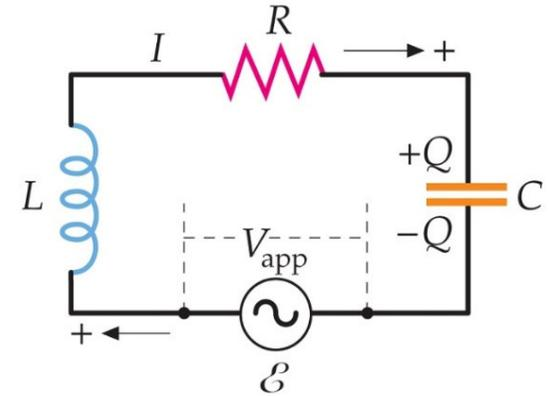
$$I_{\max} = \frac{V_{\text{app}}}{Z} = \frac{V_{\text{app}}}{\sqrt{R^2 + (X_L - X_C)^2}} = \frac{V_{\text{app}}}{\sqrt{R^2 + \left(L\omega - \frac{1}{C\omega}\right)^2}}$$
