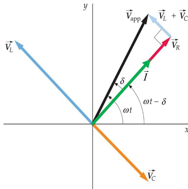
$$Z = \sqrt{R^2 + (X_L - X_C)^2} \Rightarrow V_{\text{app}} = ZI_{\max} = \text{Re}(Z^*)I_{\max}$$
